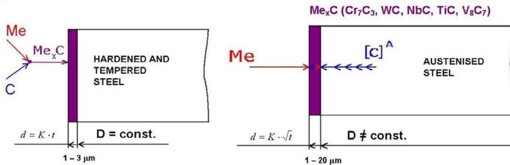
Figure 1. Schematic presentation of the basic difference between the processes of coating and diffusion carbide layer formation
