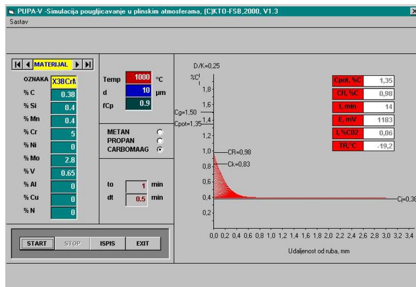
Figure 3. Program interface for the calculation of pre-carburisation parameters for the introducing of carbon required for the formation of a carbide layer of required thickness (10 µm)
