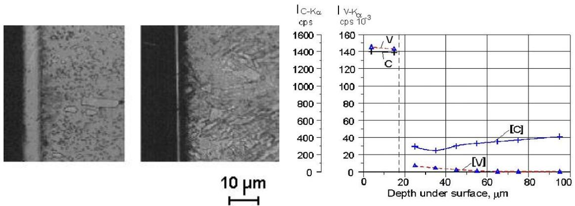
Figure 2. Metallographic cross-sections of different steels vanadised in the same conditions and the qualitative microanalysis of partial de-carburization beneath the carbide layer
